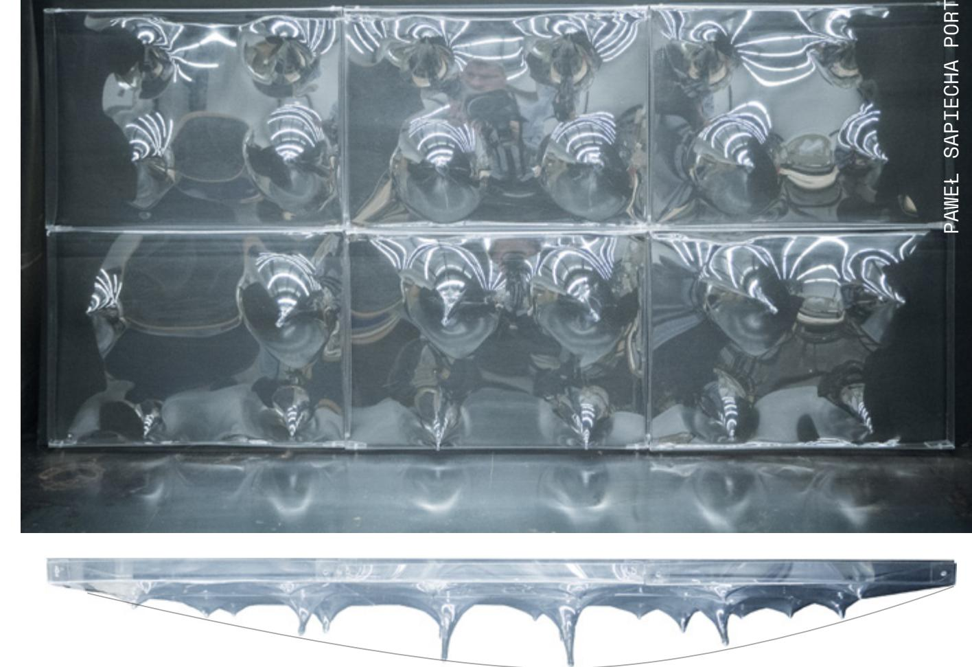
During the exercise the shape of the building's front facade was optimized with the use of a genetic evolutionary algorithm, that decreased the sun exposure by 16% in comparison to the original facade. The perforation was adjusted to the radiation map of the facade. The final model - Liquid - is a research project, that combines rapid robot prototyping with modeling thermoplastics. The spikes of the final model follow the curvature of the optimized front facade.
